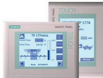
Figure 1-4 Operator and Touch Panel Displays
